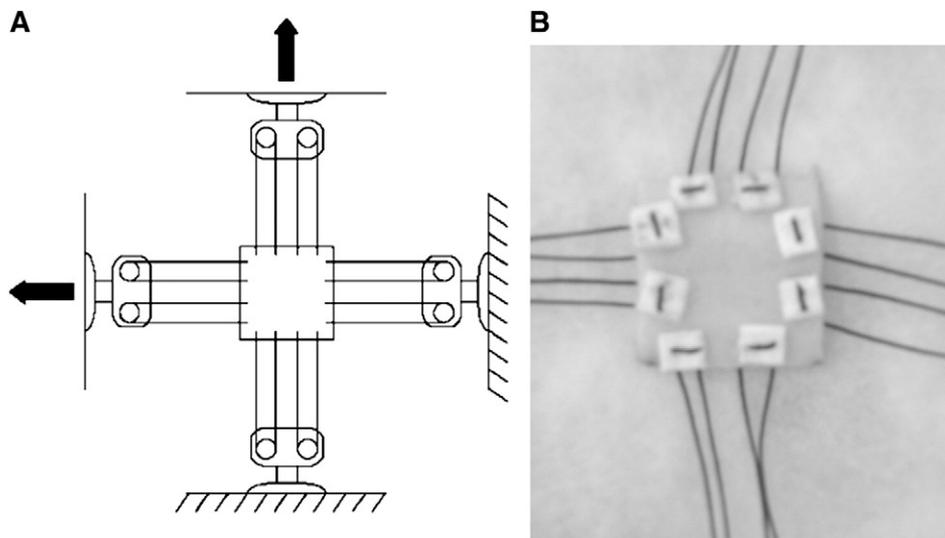
Fig. 2. (A) Schematic of the biaxial mechanical tests. (B) Picture showing the sutures and pledgets used to attach the samples to the biaxial tester.
